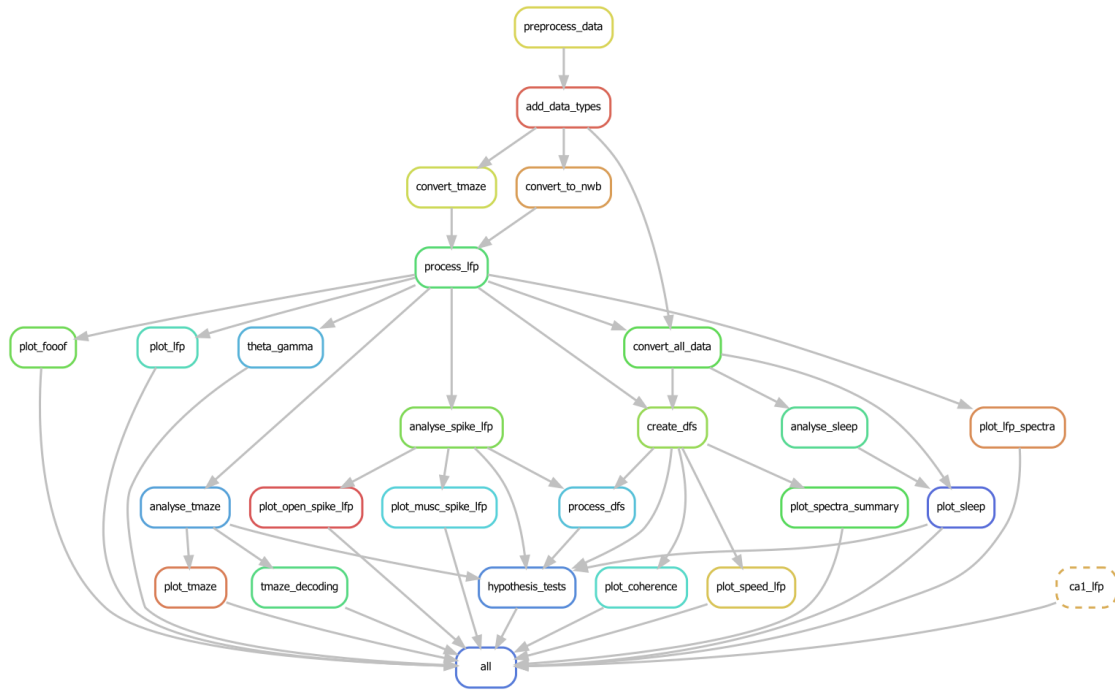
FIGURE 3.3: Combining Simuran and Snakemake to create an analysis pipeline with branching paths via directed graphs.
