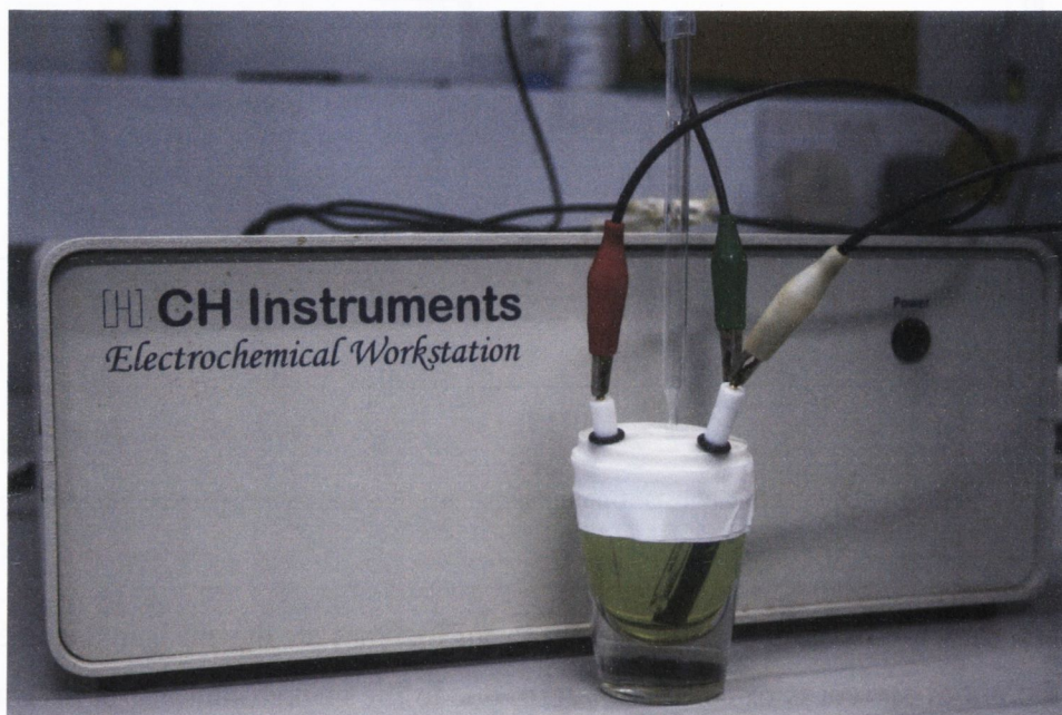
Fig. 2.6 The electrochemical cell used in the present work, along with three electrodes and a nitrogen inlet. Behind it is the CH Instruments potentiostat.
