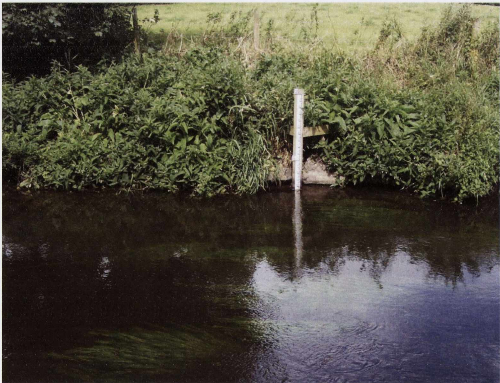
Figure 3.5d. View of the water level gauge at the water quality sampling point on the Halfcarton river in the Lough Sheelin catchment. Spot readings of water level and quality were taken by the IFI three times a week
