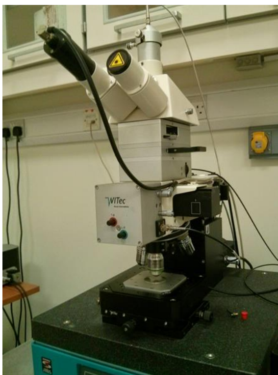
Fig. 2.11 Photograph of the WITec Alpha 300R scanning Raman and PL spectrometer used in this thesis.
