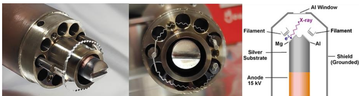
Fig. 1.12 Photographs of a dual X-ray source used in a non-monochromated XPS system here, alongside a representation of the various components of a standard source. 71
