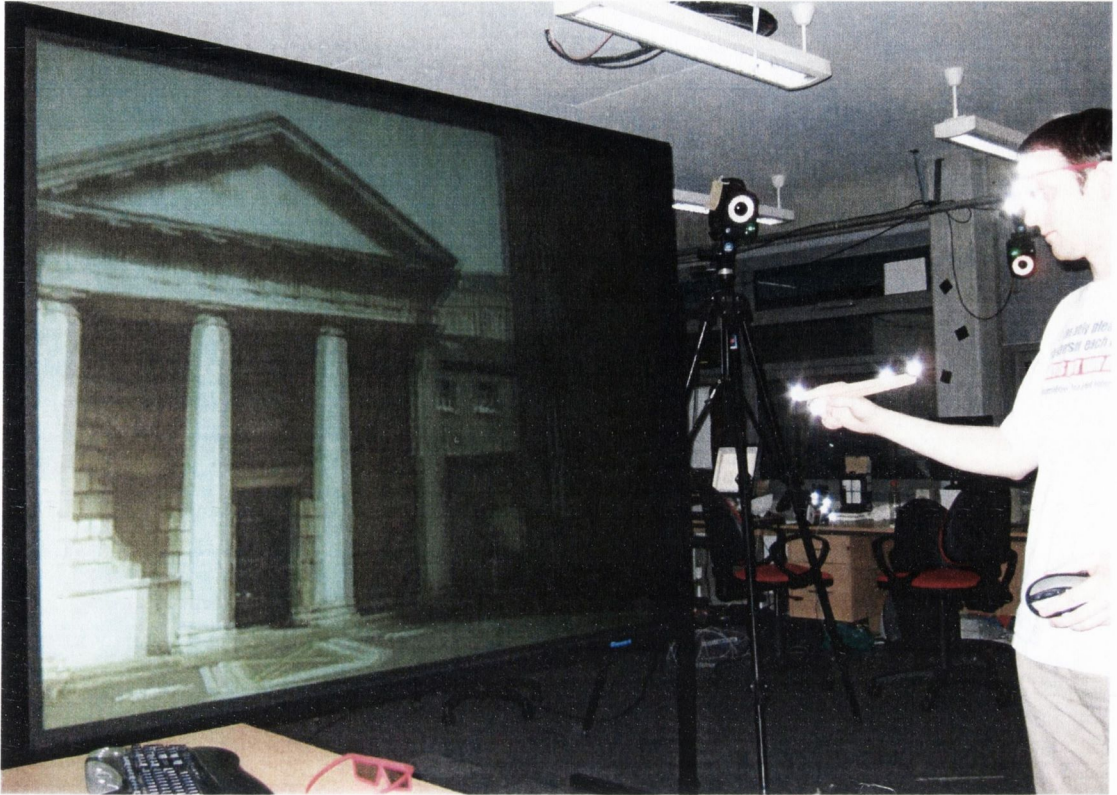
Figure 4.9: System setup. Two of the Vicon cameras can be seen in the background. The bright glares are the reflective markers.
