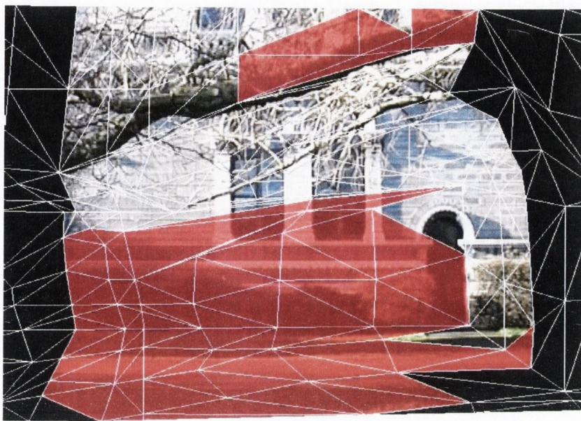
Figure 6.11: An input view of the Exterior scene after processing: the geometric proxy is drawn in white. Triangles in black belong to vertex rings that contain a triangle that is not fully visible in that view, which makes them unusable in the first place. Triangles in red belong to sub-views that were discarded by our technique.
