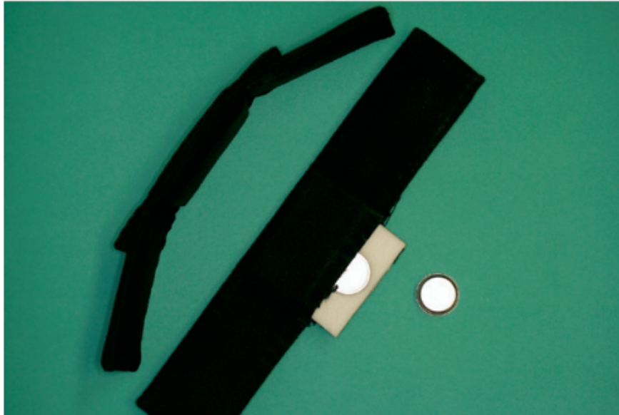
Figure 6: The Thermochron i-Button sensor used by Bos et al. to examine subjective and objective reports on compliance with headgear therapy (Thermochron i-Button, DS1921G; Maxim Integrated Products, Sunnyvale, Calif) (Bos et al., 2007).
