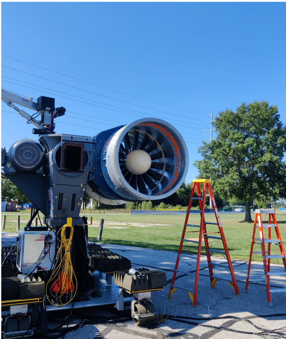
b) T-Liner installed in ANCF at the White Field test facility
