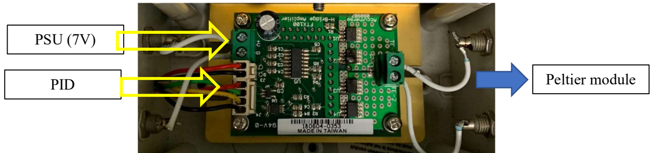
Figure 4.13 The H-bridge (FTX100) is connected to the PSU and PID controller.
