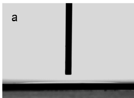
Figure 5.2 Toluene static contact angle on \text{SiO}_x . 21
