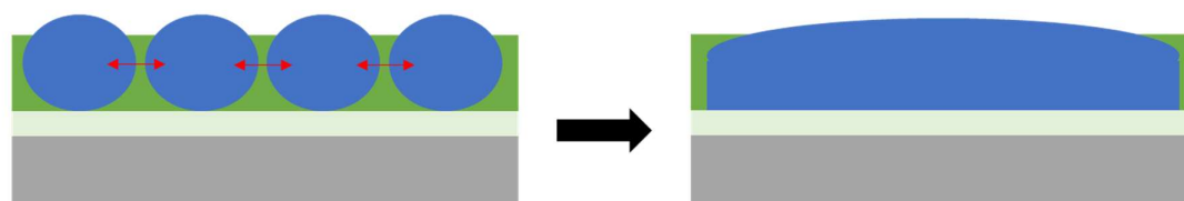
Figure 6.50 Effect of water droplet interaction during a coalescent event 16
