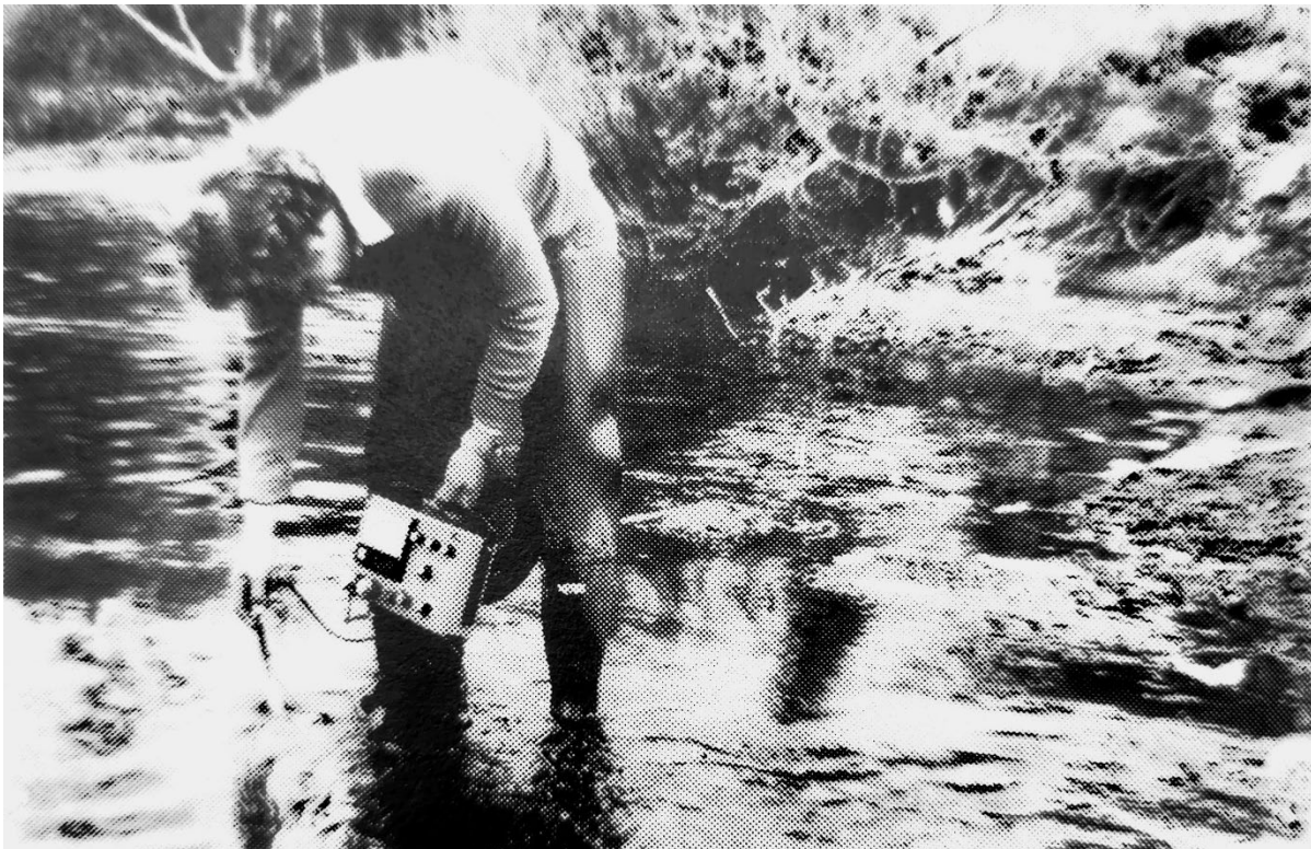
Figure 4.3: An instructional image showing proper technique and river position for measuring dissolved oxygen at the site of a fish kill. Source: Boelens and O’Sullivan, A Guide to the Investigation of Fish Kills , 6.
