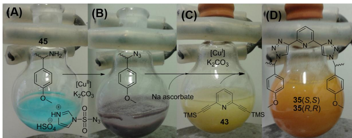
Figure 1.30 Schematic representation of the one-pot diazo-transfer-deprotection-'click' reaction for the synthesis of ligands 35R/S utilising the colour changes to monitor reaction progress. 156
