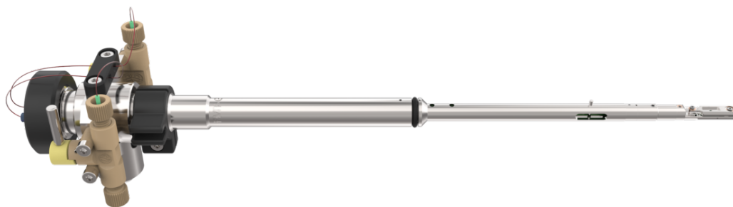
Figure 19: DENS Solutions Climate Specimen Holder. (Courtesy of DENS Solutions, Delft, Netherlands.)
