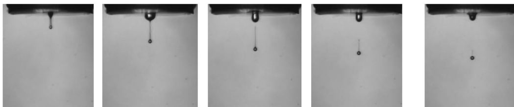
Figure 26: Time series photographs of the ejection of a pristine droplet from the printhead nozzle.
