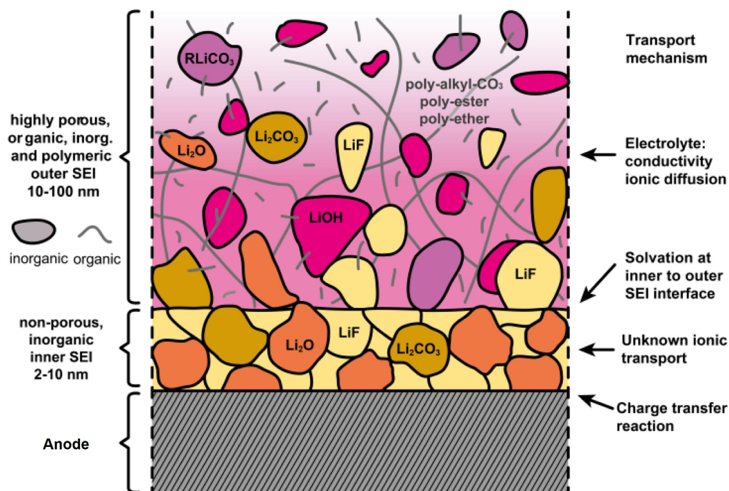
Figure 5: Schematic depiction of the SEI at an anode interface, and ionic transport within the SEI.
