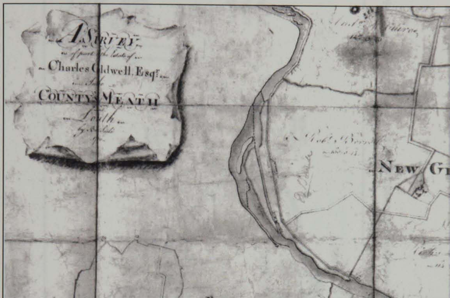
Fig.5.6: Detail from 'A Survey of part of the estate of Charles Caldwell, Esq. in the County of Meath and Louth with names of tenants, by Bernard Scalé, 1766', showing the two canals at Broe. The innermost cut to the east is for the new navigation and the outermost is for the millrace to Broe mill. NLI, Manuscript map, folder 21.F.78.
