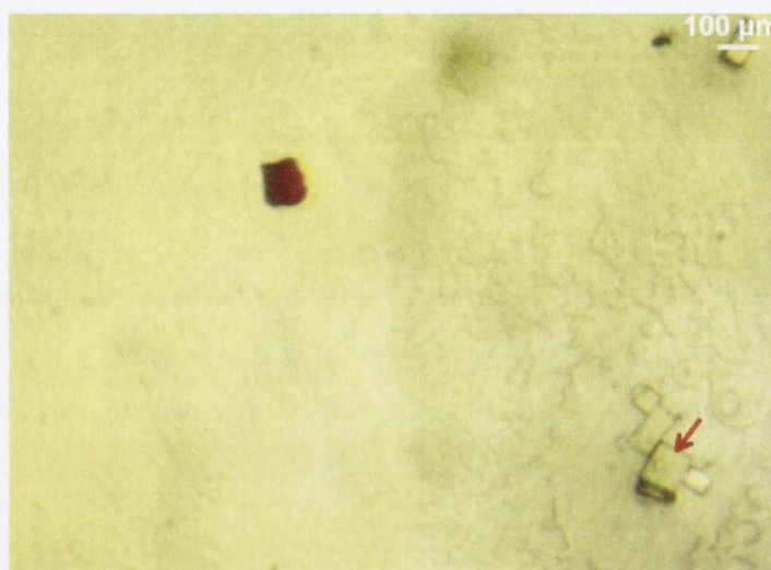
Figure 3.11. Example of in situ salt crystals obtained in the bicelle crystallization trials at 20 °C.
