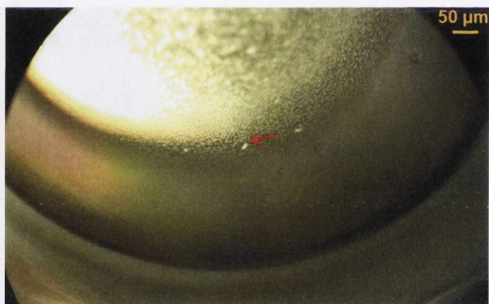
Figure 3.26. In surfo optimized crystals of LysP/nanobody CA5755 complex.
