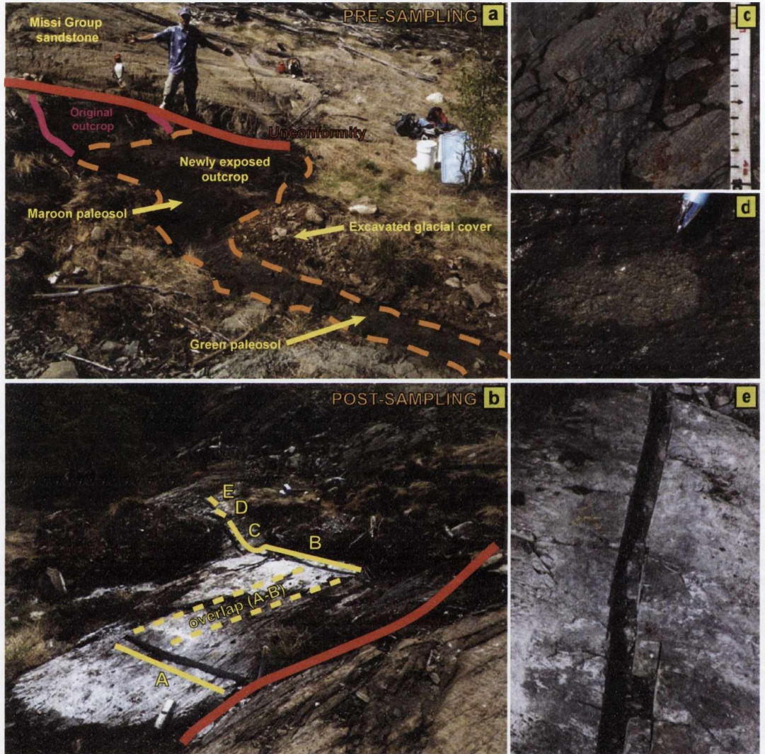
Figure 3: Outcrop of the Flin Flon paleosol excavated and sampled for the present study (UTM: 14U 0316989 mE, 6070745 mN): a) View of the full profile looking approximately NW showing the area of outcrop originally exposed prior to new excavation and sampling, the unconformity with the overlying Missi sandstone, and the colour of the paleosol (note the change between maroon and green paleosol); b) View of the full profile looking approximately SE from the Missi sandstone, showing the continuous channel and separate sections (A-E) created for geochemical sampling. Note the offset in the profile sections between A and B; c) Secondary dolomite in the B horizon of the paleosol; d) Green corestone in the maroon paleosol at a depth of 90 cm (Section A); e) Channel for Section A. Channel is approximately 10 cm wide.
