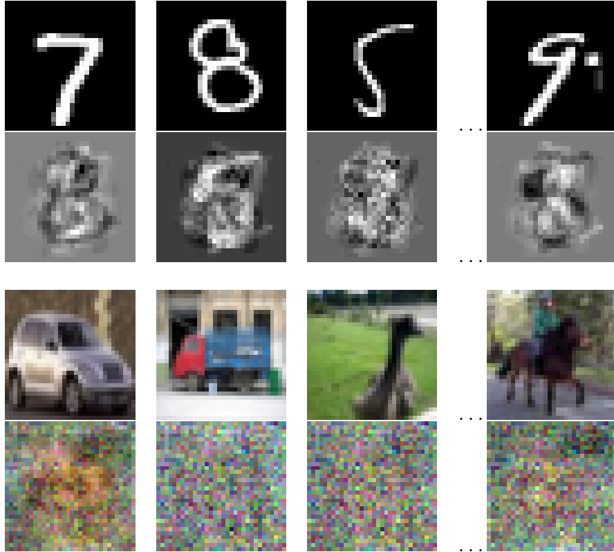
Figure 4.12: A mini-batch from MNIST (top) and CIFAR10 (bottom) and distinct forged counterpart produced by our error matrix sampling approach. Both examples produce an approximation error on the order of 10^{-7} , 5 orders of magnitude smaller than existing attacks.
