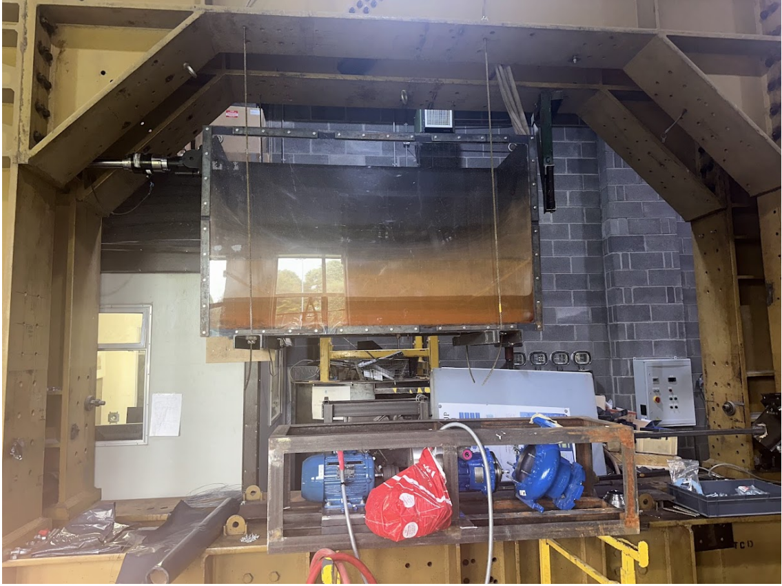
Figure 7.4: Full-scale TLD tested in the MTS real-time hybrid test system at Trinity College Dublin, Ireland
