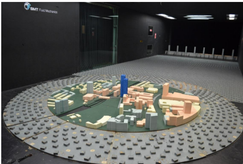
Figure 4.7: Wind tunnel set up showing scaled model of Ten Degrees in blue and the surrounding conditions
