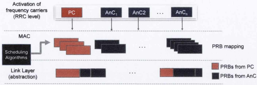
Fig. 5.4 HetNet+ uses existing link models and scheduling algorithms
