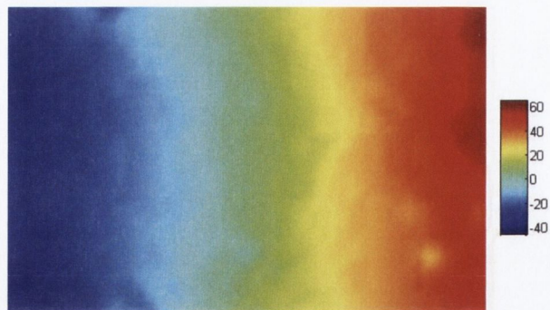
Figure 8.13 – Typical cross-fibre direction sample raw displacement as recorded by DIC code.
