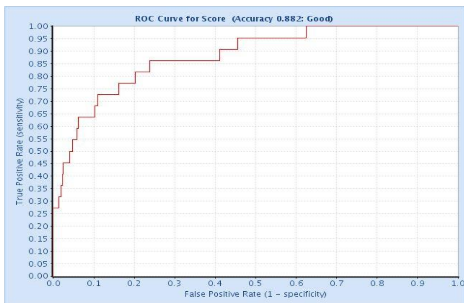
Figure 3.41. Shows the ROC-AUC curve with a score of 0.88. The x-axis shows rate of false positive, and y-axis shows rate of true positives.
