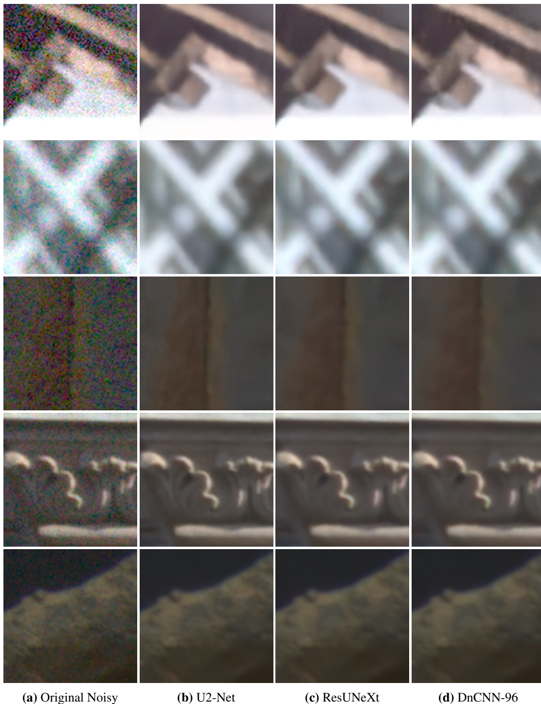
Fig. 3.6 Denoising results from the original DND benchmark, showing 128×128 crops of denoising outputs. From left to right: Original Noisy, U2-Net, ResUNeXt, DnCNN-96.
