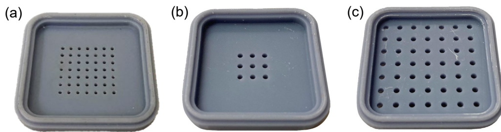
Figure 4.19: 3D printed orifice plates for (a) baseline, (b) SOO and (c) MOO designs.
