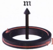
Figure 2.1: The equivalence of a circulating current \mathbf{I} and a magnetic moment \mathbf{m}
