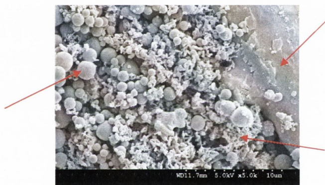
Figure 6.6 SE micrograph of trypsin:trehalose spray-dried in a mass ratio of 1:1 from 98% EtOH, 40% of t.s.c. AC, inlet temperature 78 °C – comp1.
