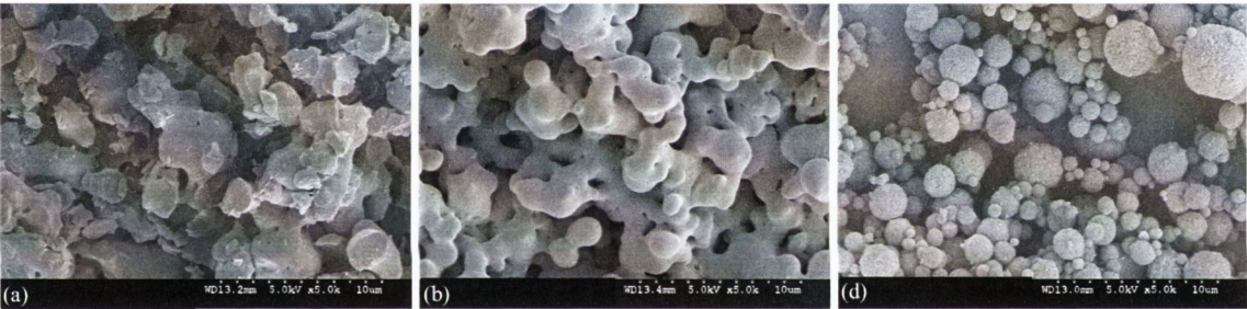
Figure 5.50 SE micrographs of composite particles taken after 24 hour storage at 25 °C/60% R.H. of (a) lysozyme:trehalose (1:4) (b) lysozyme:raffinose (1:4) (c) lysozyme:HP- \beta -CD (1:4).
