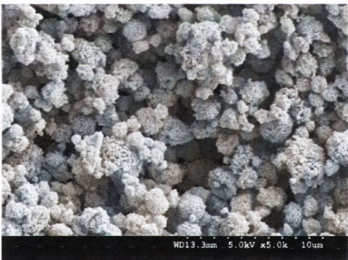
Figure 4.26 SE micrograph showing raffinose spray-dried from 79:19:2 MeOH:BA:H 2 O, inlet temperature 100 °C, 1% t.s.c..
