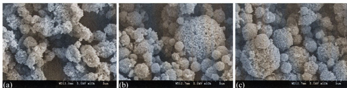
Figure 4.7 SE micrograph showing trehalose spray-dried from MeOH:BA in solvent ratios of (a) 90:10, (b) 70:30, (c) 60:40.
