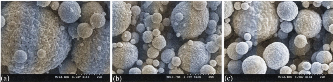
Figure 5.37 SE micrographs showing lysozyme:raffinose spray-dried at a mass ratio of 3:7 (a) using a regular cyclone (b) using a HP cyclone, and at a mass ratio of 1:1 (c) using a HP cyclone.
