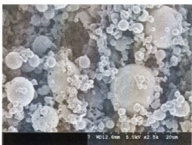
Figure 4.35 SE micrograph showing raffinose spray-dried with coumarin-6 from 60% EtOH.
