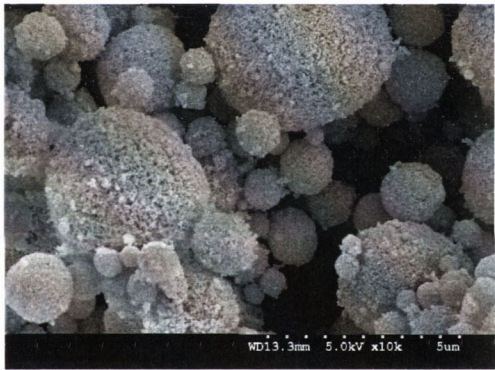
Figure 4.57 SE micrograph of Trehalose:HP- \beta -CD (ratio 1:1) spray-dried from MeOH:BA 80:20, inlet temperature 100^\circ\text{C} .
