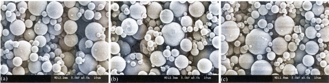
Figure 4.27 SE micrographs showing raffinose spray-dried from H 2 O, t.s.c. 2.5% and inlet temperatures (a) 110 °C (b) 120 °C (c) 130 °C.
