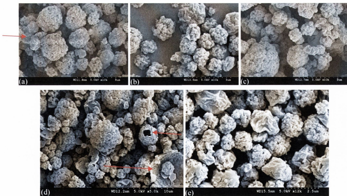
Figure 5.1 SE micrographs showing lysozyme:trehalose composite particles, spray-dried at a mass ratio of 1:1, % EtOH, % of t.s.c., inlet drying temperature as (a) 80%, 10% AC, 78 °C, (b) 70%, 10% AC, 78°C (c), (d) 70%, 10%, 90 °C (e) 70%, 25%, 90 °C; Note magnifications differ.
