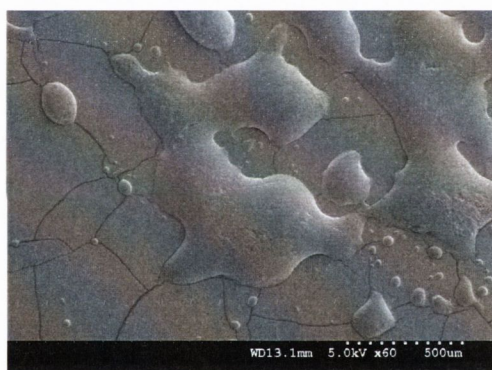
Figure 4.38 SE micrograph of spray-dried trehalose particles showing deliquescence.
