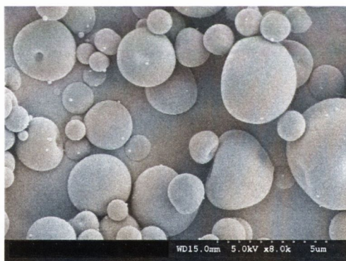
Figure 3.21 SE micrograph of lysozyme spray-dried from 80% EtOH, inlet temperature 78 °C, pH of water component adjusted to pH 8 using 1M KOH.
