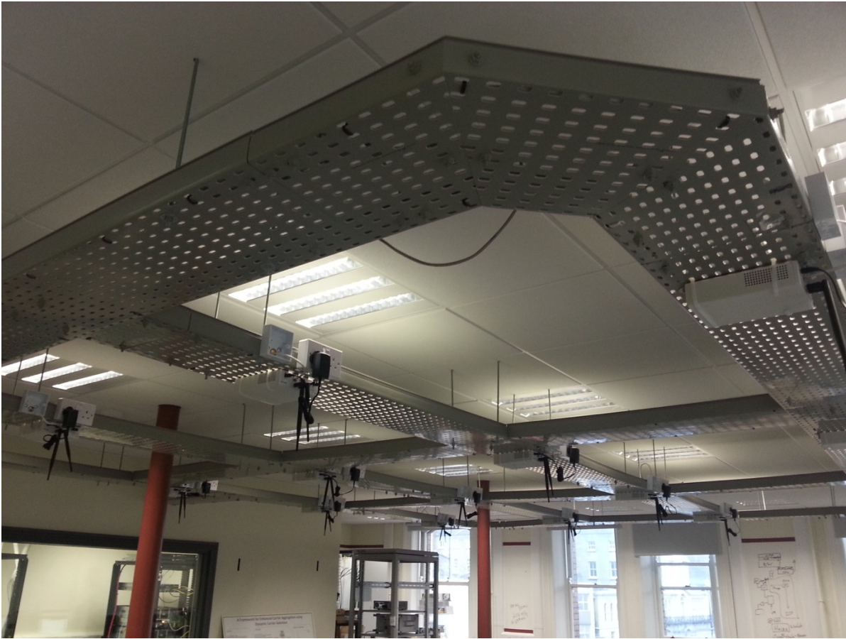
Figure 7.1: The CONNECT testbed. 16 ceiling-mounted RF front-ends are paired with virtual nodes running software radios. Virtual nodes can be reserved using an automated website and accessed remotely through Secure Shell (SSH).
