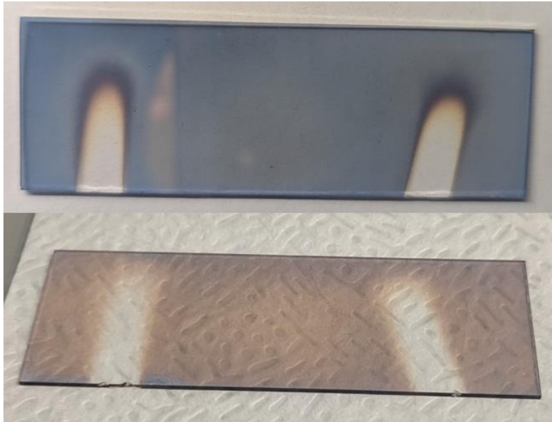
Figure 5-20 Silver dewetting visual confirmation Top: 10 nm thick silver on a glass slide, Bottom: Silver on a glass slide after being heated to 250° C
