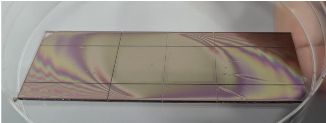
Figure 5-17: Spun on photoresist, the photoresist gets thinner near the edges.
