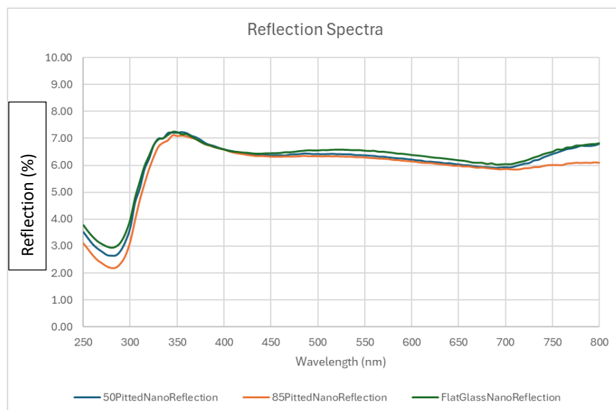
Figure 6-10: Reflection Spectra for the nanopillars, ignore the absolute values of transmission, that is a calibration issue related to using glass samples of different sizes
