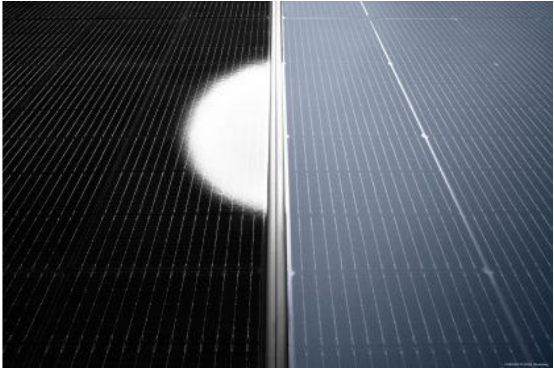
Figure 1-17 Anti-glare coating. This figure compares an ordinary solar panel with a porous silica AR coating with another solar panel with a biomimetic rose petal pattern imprinted onto a polymer layer. This Anti-glare surface was produced by Phytonics, which is a spin-off from the Karlsruhe Institute of Technology (KIT) 14
