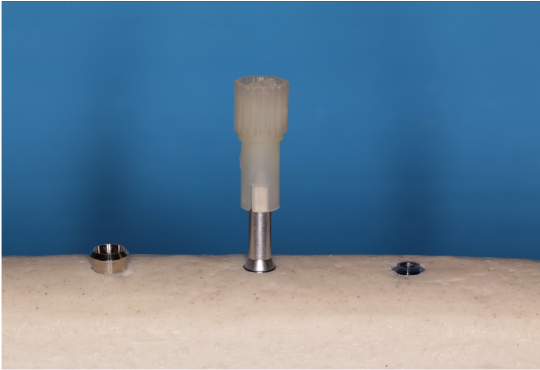
Figure 7 Photograph of SmartPeg tightening by the novel SafeMount
