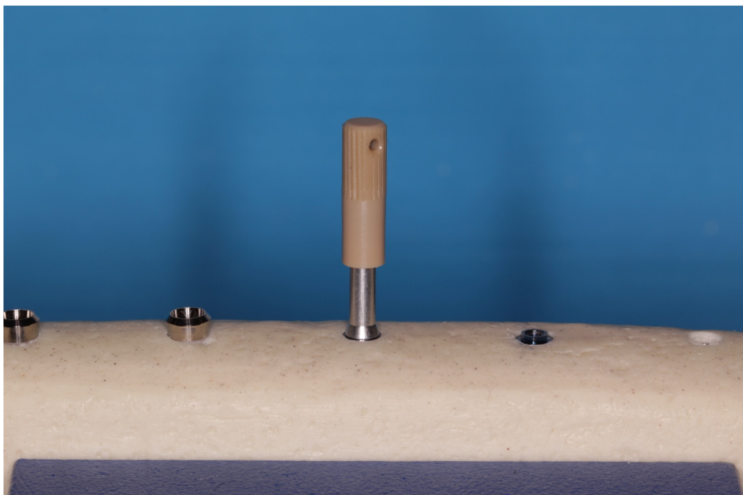
Figure 6 Photograph of SmartPeg tightening by plastic torque wrench
