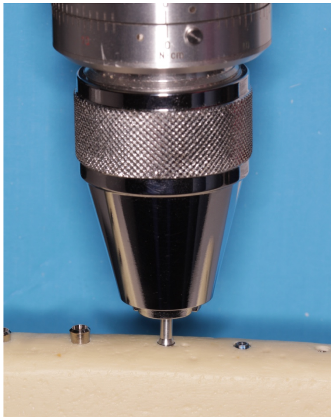
Figure 8 Photograph of SmartPeg tightening to 6 Ncm by a calibrated torque wrench
