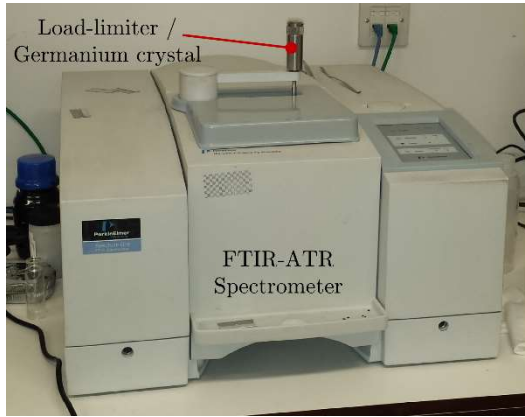
Figure 4.40: FTIR-ATR Perkin Elmer Spectrum One spectrometer specifications
