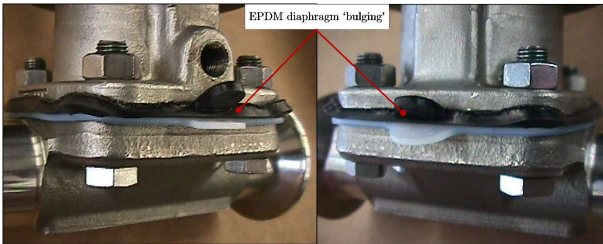
Figure 5.5: EPDM diaphragm 'bulging' due to over-torqueing
