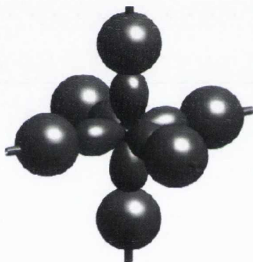
Fig. 1.6 Octahedral coordination of oxygen ion by cations showing overlap between metal s and O 2 p states (from Ref. 30).
