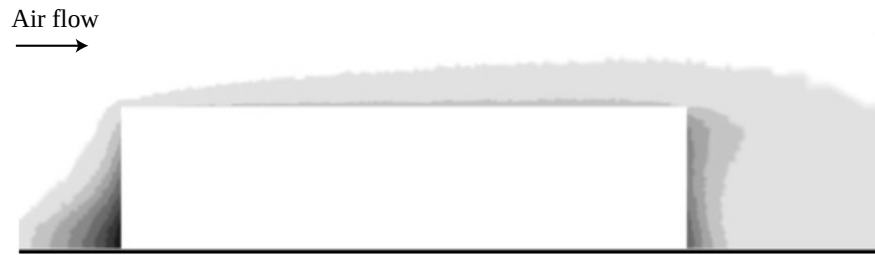
Figure 2.12: Vapour concentration ( \text{mol}/\text{m}^3 ) field surrounding a rectangular drying solid during the falling-drying rate period [77]. The greyscale ranges from 6.05 to 6.20 \text{mol}/\text{m}^3 .
