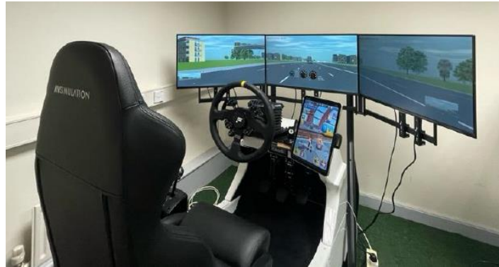
Figure 4. 1. Driving Simulator at Trinity College Dublin with a mounted Samsung Tablet.
