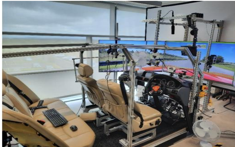
Figure 5. 2. High Fidelity dynamic driving simulator at Tobii.
