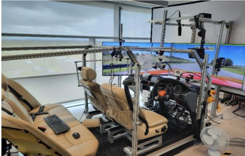
Figure 3. 3. The Driving Simulator used in Experiment two.
