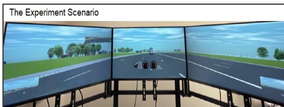
Figure 5. 3. Driving virtual environment of the simulator from SCANeR software.
