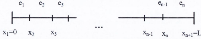
Figure 2.10: Discretisation of domain into elements e_k and node points x_k .
