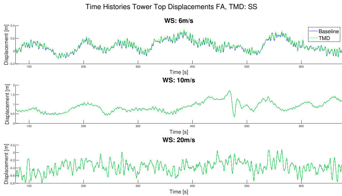
Figure 6.6: Fore-aft tower top displacements with TMD
