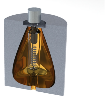
(d) 3D view of the optimised reflector and QTH lamp.
