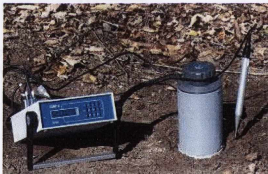
Figure 2.6: EGM – 4 CO 2 gas analyzer and SRC – 1 soil respiration chamber. Source: PP Systems.
