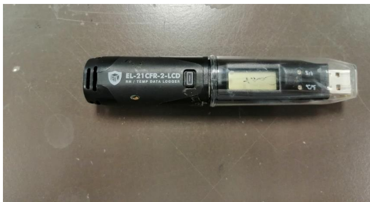
Figure 2.9: Sensor used to monitor air humidity.
