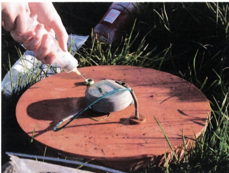
Figure 4.1. Extraction of gas samples, for \text{N}_2\text{O} and \text{N}_2 concentration and isotopic composition, from the static chambers used in the study.
