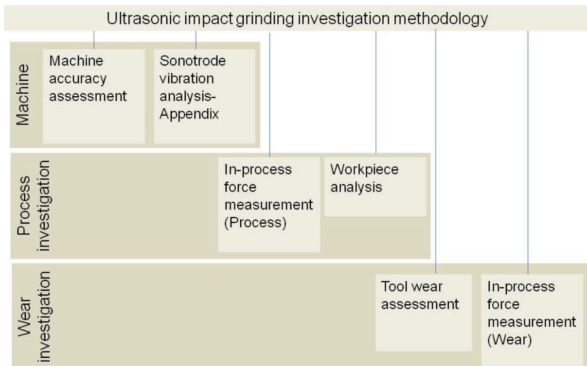
Figure 4-1: Ultrasonic impact grinding investigation methodology showing investigations in 3 phases of machine, process and wear.
