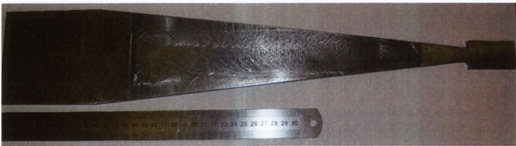
Figure 5.3: Finalised SAWR calibration beam manufactured on Mild EN-8 steel
