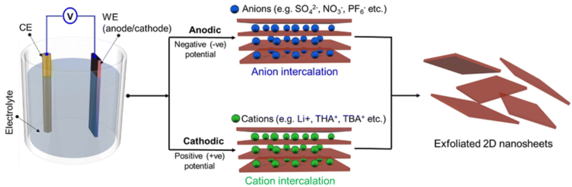
Figure 1.14: Schematic of Electrochemical Exfoliation. The setup includes two electrodes, an electrolyte, and a voltage source. TMD crystals are used as the working electrode, and depending on the chosen electrolyte, ions are forced to intercalate between the van der Waals layers of the crystal, causing expansion and leading to easy exfoliation [116].
