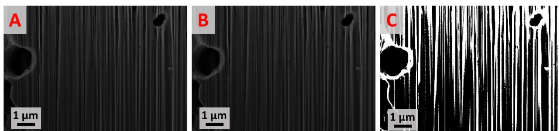
Figure A2.15. ImageJ processing summary. A. Raw SEM image. B. after median 3D filter. C. Binarised image.
