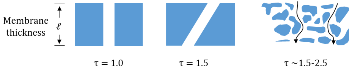
Figure 1.6. Cross-section of membranes showing varying tortuosity. Adapted from Baker (2012). 72
