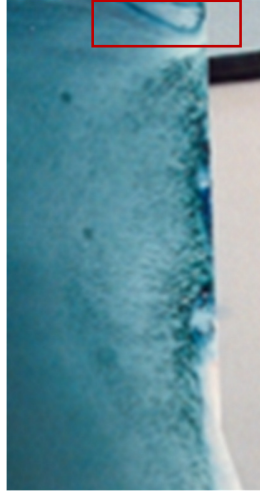
Fig. 15 Wing body junction flow visualization results top-down view ONERA wind tunnel test.
