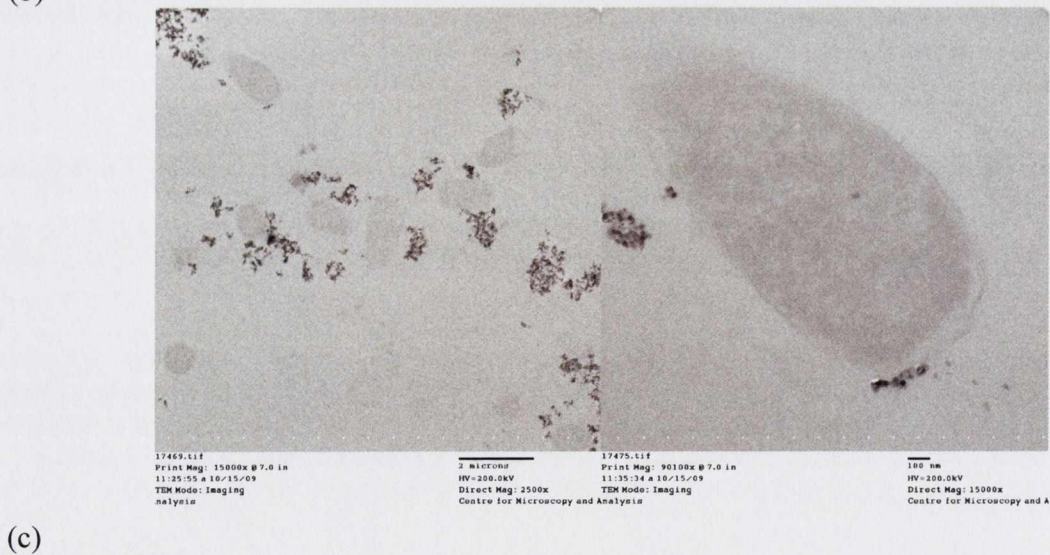
Figure 4.5 TEM images of bacteria (a) after 15 h illumination - no \text{TiO}_2 ; (b) before treatment - 50 mg/L \text{TiO}_2 ; and (c) after 15 h illumination - 50 mg/L \text{TiO}_2 .
