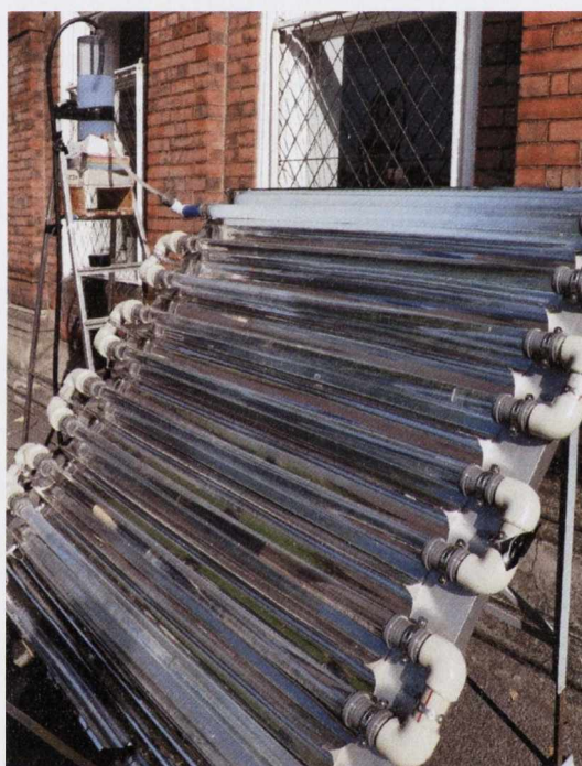
Figure 3.3 Full-scale CPC during mixing of \text{TiO}_2
