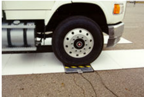
Figure 1.2: Road-based capacitive mat weight sensor [13]
