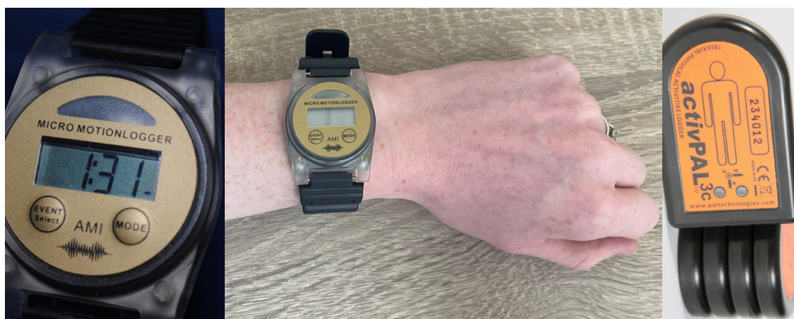
Figure 6. Accelerometry devices used within the study. Left: The Ambulatory Monitoring Inc. Micro Motionlogger wrist accelerometry device with event button on the left below the time. Middle: Micro Motionlogger in situ. Right: activPAL3™ thigh accelerometry device.
