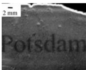
Figure 1.21: Fluorescence image of a pattern generated on 9,10-diphenylanthracene monolayer; reproduced from ref. 228. 228
