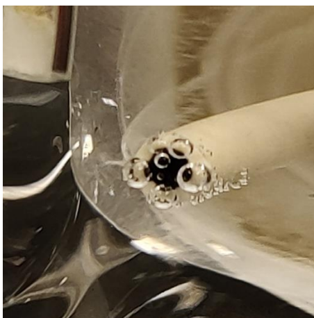
Figure 4.23: Bubble formation on electrode surface.
