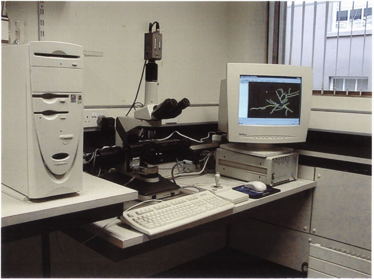
Figure 3.2 Apparatus used for quantitative morphometric analysis of intracellularly filled medium-sized densely spiny striatal neurons.
