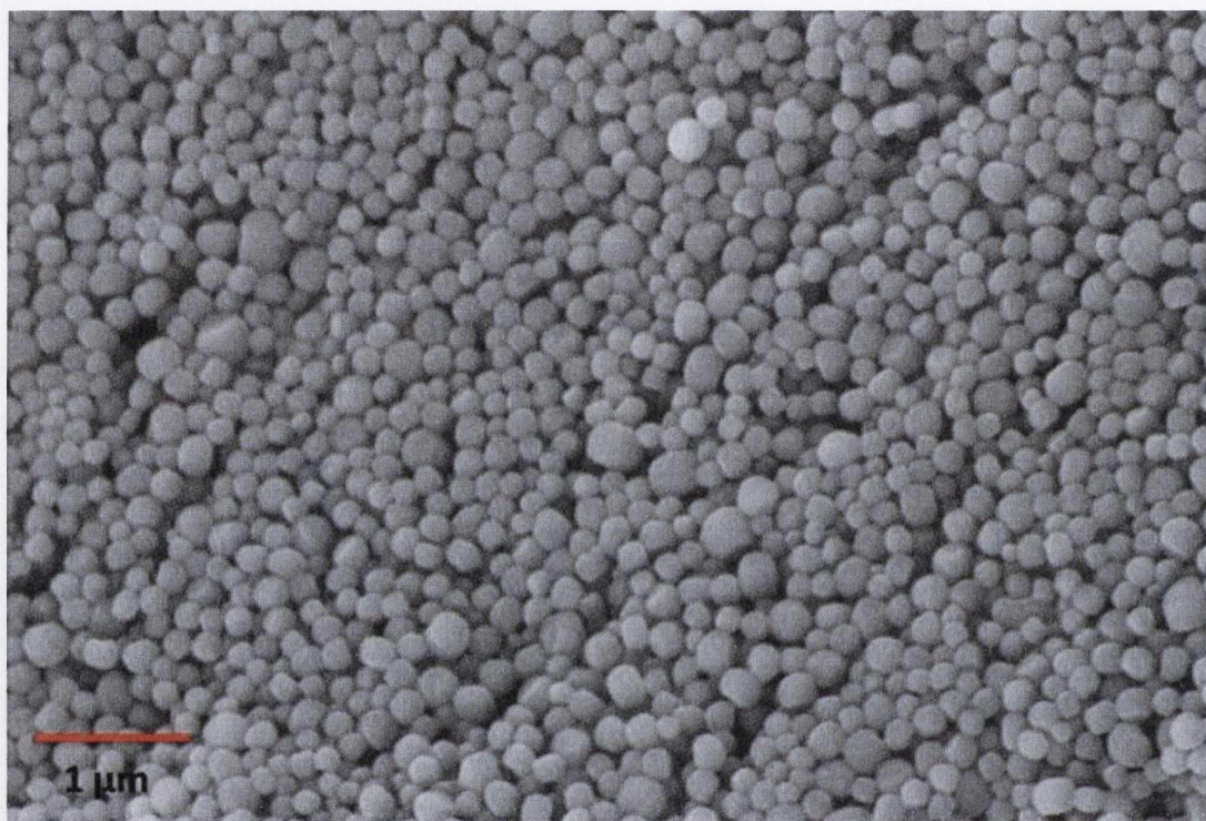
Figure 3.10. SE micrograph of freeze dried ITR NPs precipitated using 1 mg/ml Poloxamer 407 in the solvent phase at 80°C.
