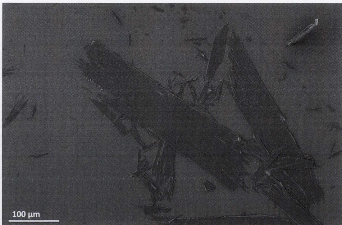
Figure 4.18. SE micrograph displaying the fragility of CH sh as can be inferred from the presence of fines in the sample.
