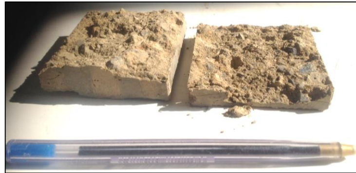
Figure 7. Shear failure of 15% cement earth specimen.
