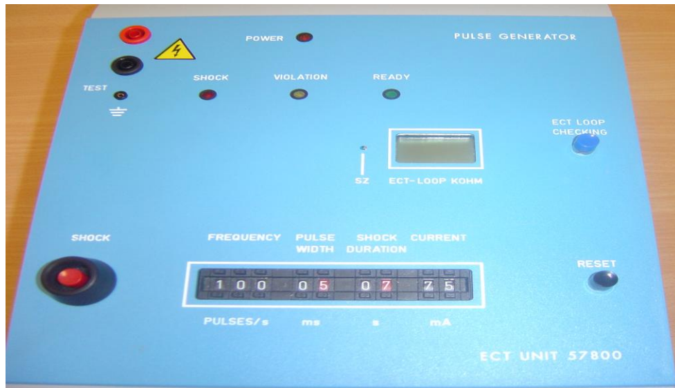
Figure 2-1 ECT unit used to administer electroconvulsive stimulation
